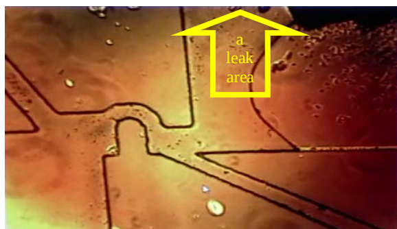
Fig. 5 Slip flow profile occurred at the middle path of the channel because of leaking next to an electrode
