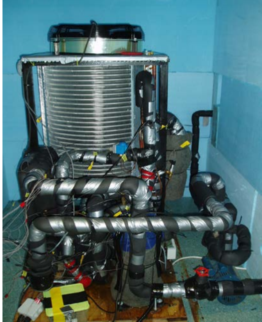
Fig. 4 Test bed of EVI heat pump
