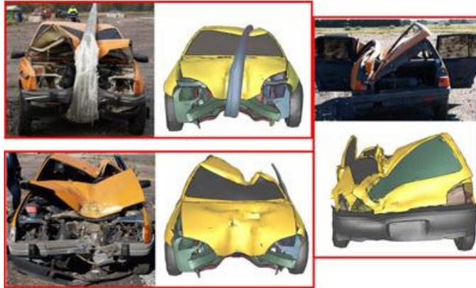
FEA of the crash-test between vehicle and lighting columns (Klyavin,2007)
