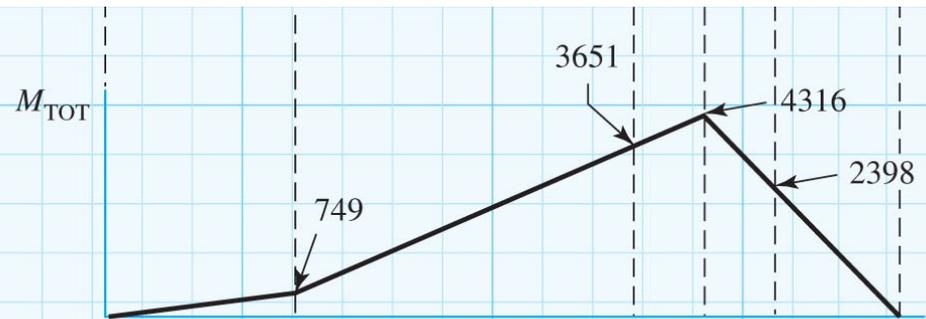
Start with point  $I$ , where the bending moment is high, there is a stress concentration at the shoulder, and the torque is present.
