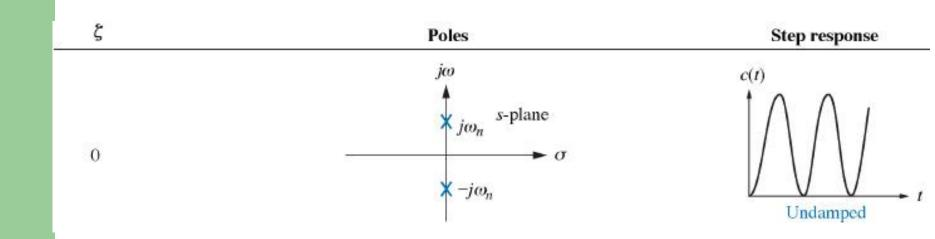
Let us begin by finding the step response for the general second-order system of Eq. (4.22). The transform of the response, C(s), is the transform of the input times the transfer function, or
