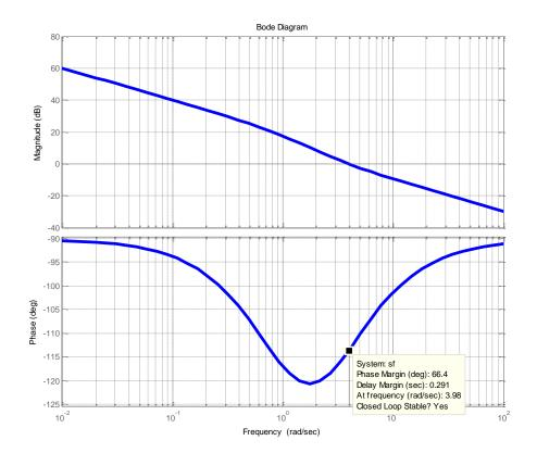
Phase margin(PM)= \_\_\_\_\_deg. at \_\_\_\_\_ rad/sec; Gain margin(GM)= = \_\_\_\_dB at \_\_\_\_\_rad/sec
