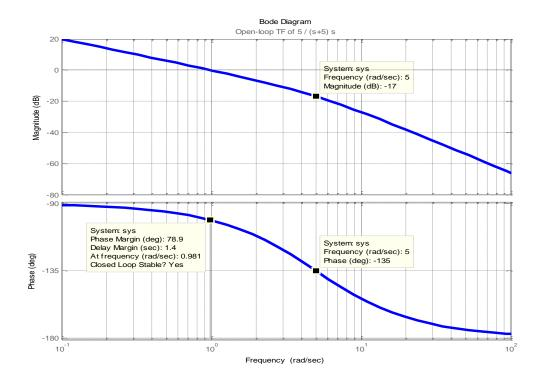
**Example** PI design; Desired system is K<sub>v</sub> of 10 sec<sup>-1</sup>, Phase margin is at least 60 degree.
