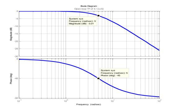
Bode diagram of open-loop transfer function is
