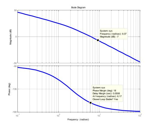
Phase margin(PM)= 18 deg. at 6.17 rad/sec ; Gain margin(GM)= =+  $\infty$  dB Step III: Phase margin requirement is 50 deg. plus 10 deg. Total PM is 60 deg.
