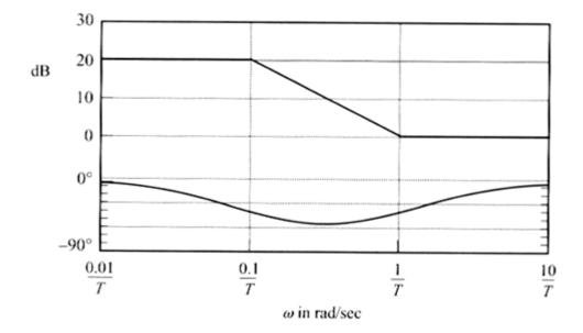
**Example** Lag design ; Desired system is K<sub>v</sub> of 16.22 sec<sup>-1</sup>, PM of 60 degree and GM of least 10 dB
