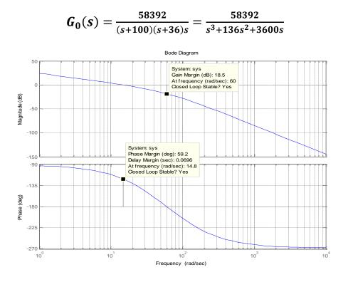
Step II: Plot bode diagram of new open-loop TF with new gain such as
