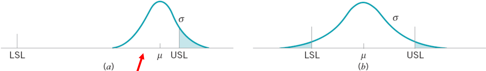
■ FIGURE 8.3 Some reasons for poor process capability. (a) Poor process centering. (b) Excess process variability.
